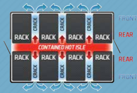
Hot-aisle containment system (HACS) deployed with row-oriented cooling
